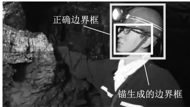
图 2 锚生成的边界框和正确边界框对比 Fig. 2 Comparison of bounding box obtained by anchor and correct bounding box
